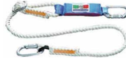
Adjustable lanyard made of polyamide, Ø 14 mm, with integrated absorber strap and aluminum alloy connectors. Length adjustment from minimum 1.10 m to max. 1.60 m. - Weight: 615 g
