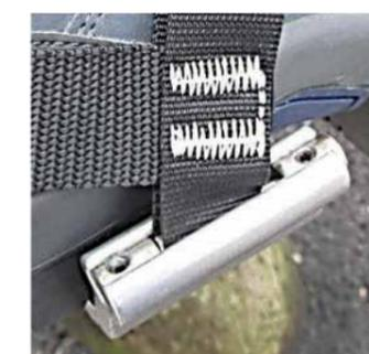
Sub-foot made of aluminum alloy, equipped with two steel teeth and hole for connecting the steel arc; depending upon the pole diameter, the operator can easily replace the arc. Straps are replaceable by unstringing them using a spanner.
