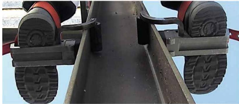
Suitable for double T-beam structures with thickness 5 to 20 mm – Foot-support of cast aluminium alloy with rubber pad polyester straps and special irons covered with anti-slip rubber hose. Weight per pair: 2,7 kg
